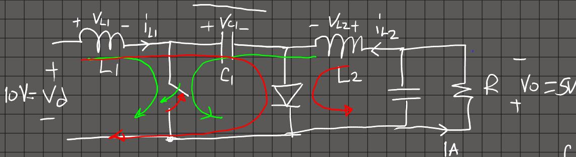
$$V_D = V_d \cdot \frac{D}{(1-D)} \Rightarrow \frac{V_o}{V_d} = \frac{5}{10} = \frac{D}{1-D} \Rightarrow D = \frac{1}{3} = 0.33 \dots$$
