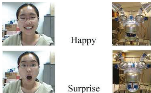
Figure 12. Human expression imitation by a robot (Ge, 2008). Detected keyframes associated to the video (left), the recognized expression (middle) and the corresponding response of the robot. With permission from © 2008 IEEE
