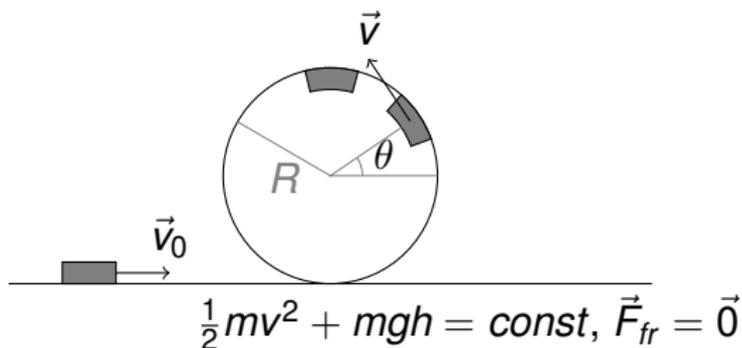
**Q:** Assume that the cart is going with a very slow speed  $v$ . What is the maximum height that it can reach on the circular track?
