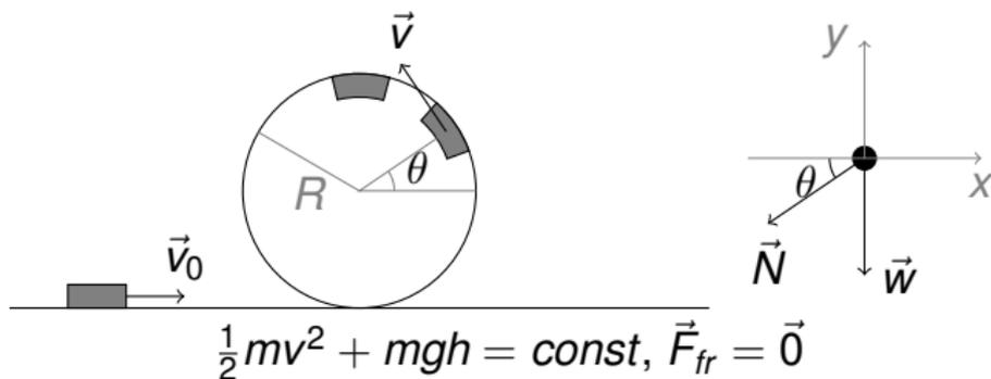
**Q:** Assume that the cart is going with a very slow speed  $v$ . What is the maximum height that it can reach on the circular track?
