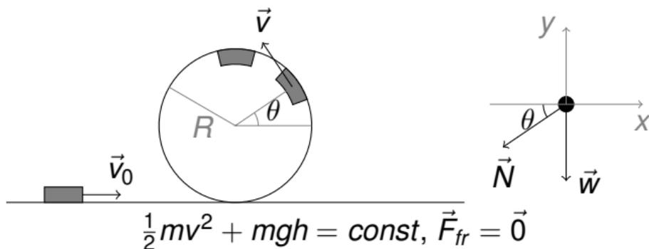
**Q:** If the cart is moving with a speed less than the minimum speed, at what point will it leave the track?
