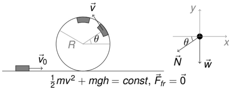
**Q:** What is the minimum speed with which the cart should have at the bottom so that it can go around the top of the loop?
