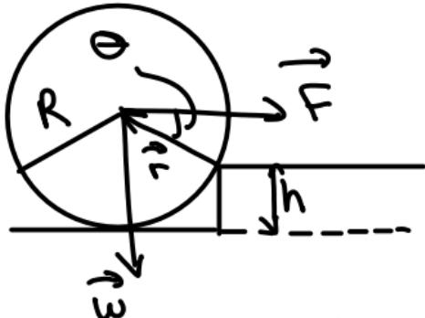
What is the minimum  $\vec{F}$  necessary to roll the sphere up the step?
