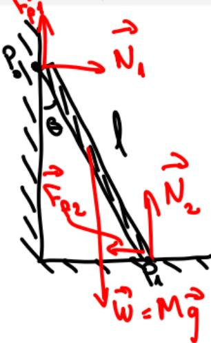
Torques with respect to  $P_0$  &  $P_1$  should be zero:
