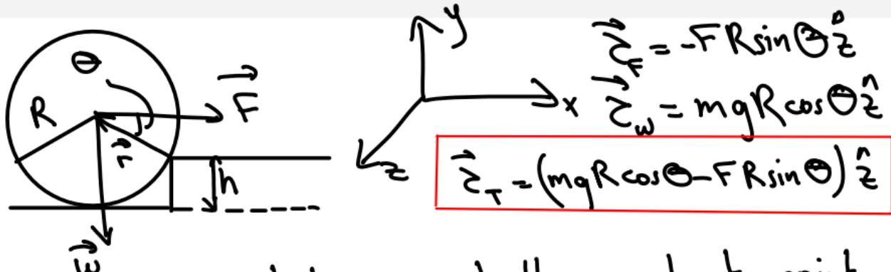
If the sphere rotates around the contact point, it should obtain an angular velocity in the  $-\hat{z}$  direction. Hence  $\vec{\Sigma}_T$  should create an angular acceleration in the  $-\hat{z}$  direction.
