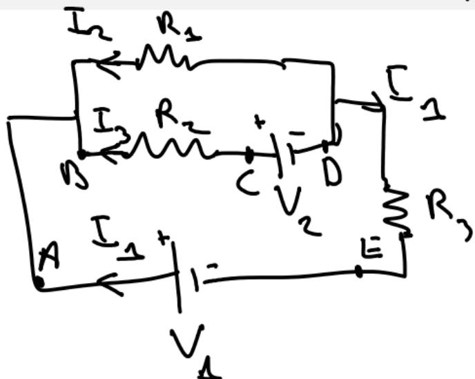
$$\begin{aligned}V_{NA} &= V_{AB} + V_{BC} + V_{CD} + V_{DE} + V_{EA} \\&= 0 - \mathcal{E}_3 R_2 + V_2 + \mathcal{E}_1 R_3 - V_1\end{aligned}\quad (1')$$
