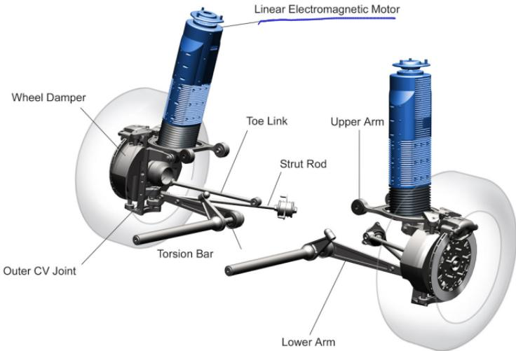
Bose suspension system, Bose suspension will be mass produced
