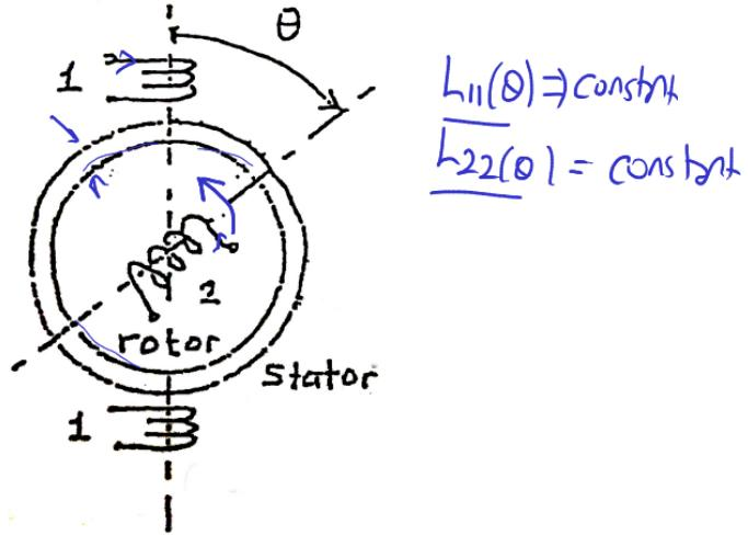
$$T = \underbrace{i_1 i_2}_{\substack{\text{will be} \\ \text{reverse}}} \frac{\partial M}{\partial \theta} : (L_{11}, L_{22} \text{ constant})$$
