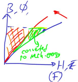
Electrical Energy = Magnetic Energy + Mechanical Energy
