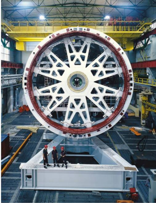
Wind Turbine Synchronous Generator (12 rpm)
