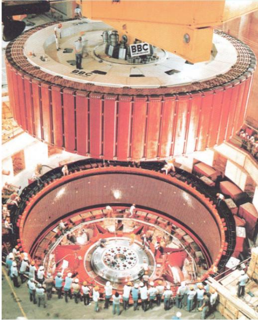
16 m diameter, 91 rpm, Rotor Mass: 2650 t
