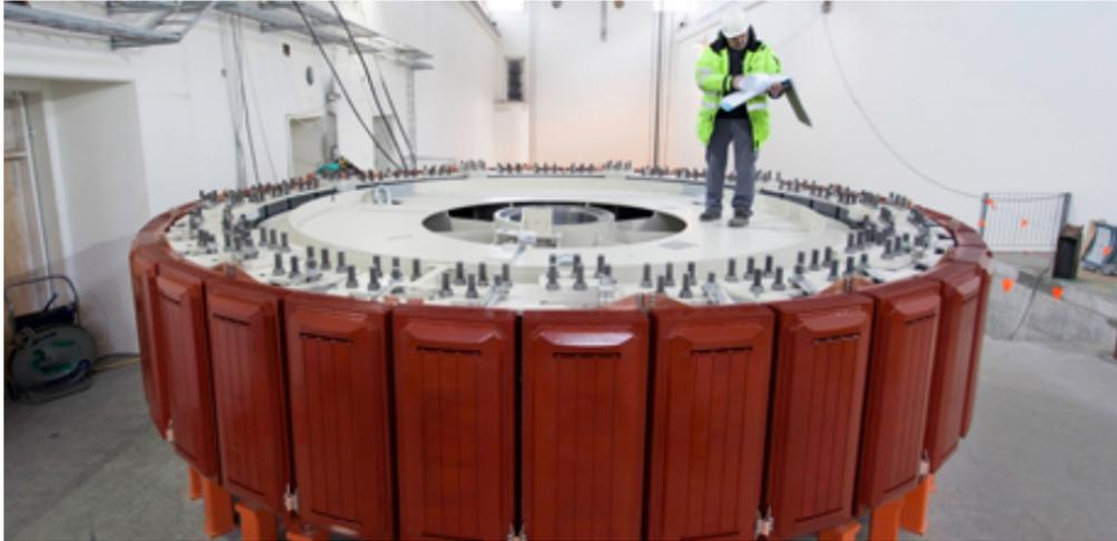
Used in large-pole low-speed generators (e.g. hydroelectric plants)
