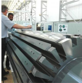
**Fig: Cylindrical rotor with slotted rotor surface along axial length to house field windings**
