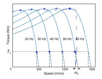
Stator voltage is varied with frequency to eliminate torque reduction  $_{\ 20\,/\,40}$
