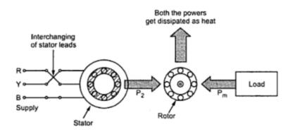
Plugging obtained by interchanging two stator phases
