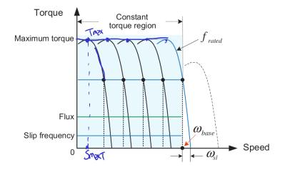
If we set the slip to the point where max torque is produced ( $s_{max-T}$ ), the machine can be accelerated quickly.
