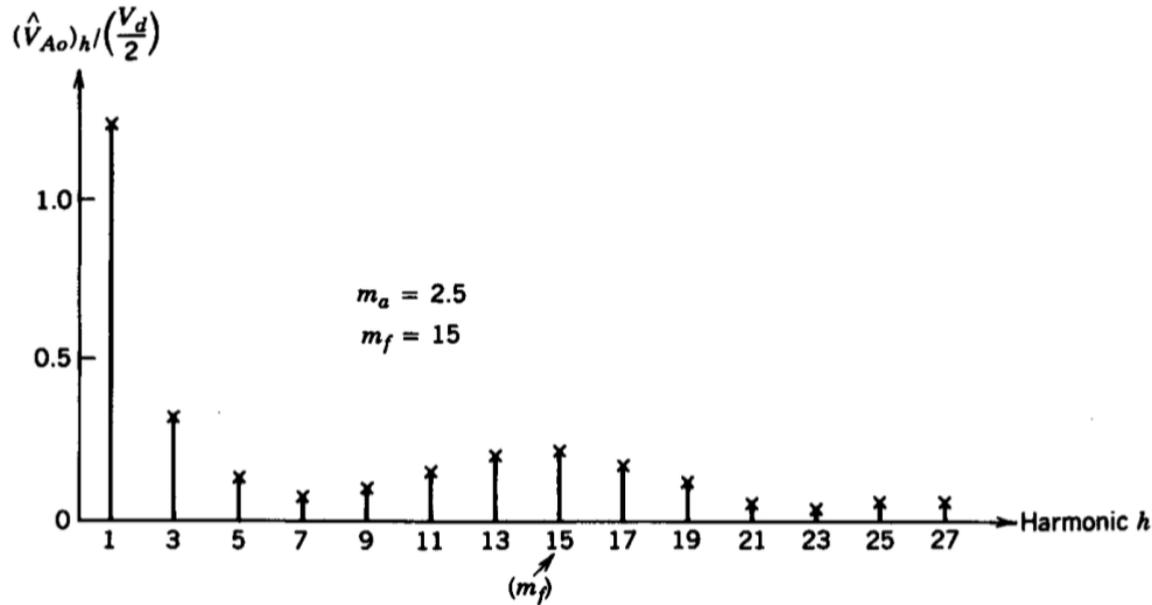
Figure 8-7 Harmonics due to overmodulation; drawn for  $m_a = 2.5$  and  $m_f = 15$ .<sup>21/50</sup>
