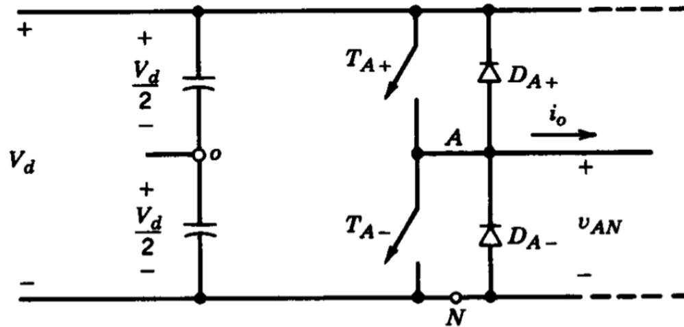
In order to have equal capacitor voltage,  $i_o$  cannot have a DC component
