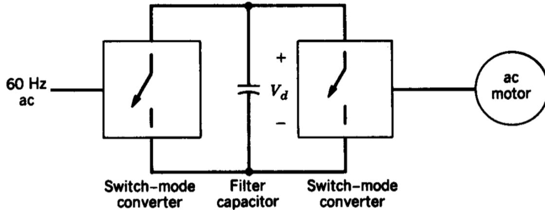
Back-to-Back Converter, Active Front-End Converter, Variable Frequency Drive (VFD)
