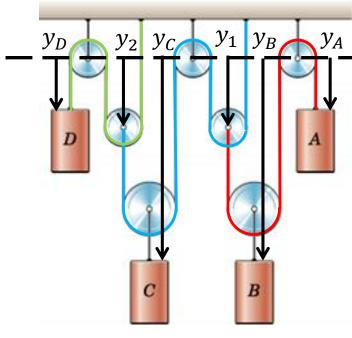
Example 2/222 (4<sup>th</sup>), 2/221 (5<sup>th</sup>), None (6<sup>th</sup>), 226 (7<sup>th</sup>), None (8<sup>th</sup>) Neglect the diameter of the small pulley attached to body A and determine the magnitude of the total velocity of B in terms of the velocity  $v_A$  which body A has to the right. Assume that the cable between B and the pulley remains vertical and solve for a given value of x.
