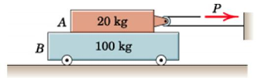
The assumption fails. Friction is not sufficient so that the two blocks can move together. Therefore there is sliding. For sliding the friction force is at its maximum value:
