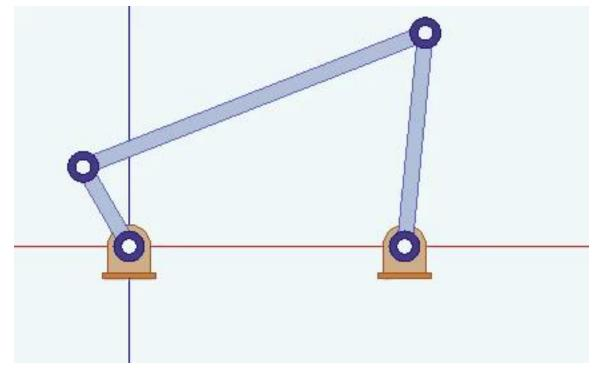
Please recognize that we have a point A on body OA (crank) that makes fixed axis rotation about O and another point A on body AB (coupler). These two points are permanently coincident points both on the axis of the pin (revolute) joint connecting two bodies. Similarly point B on body BC (follower) makes fixed axis rotation about point C and we have a permanently coincident point B on body AB.
