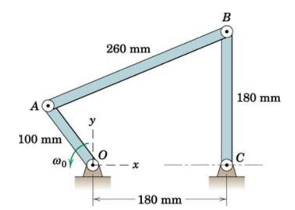
Four-bar mechanism is formed by connecting four rigid bodies (one is ground and that's why English people call it a three-bar mechanism) by four revolute (pin) joints.
