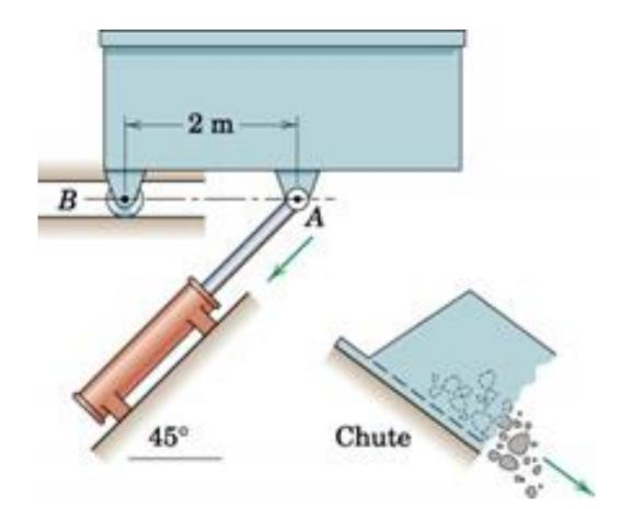
$$\begin{aligned} \vec{a}_{A} &= \vec{a}_{B} + \vec{a}_{A/B_{t}} + \vec{a}_{A/B_{n}} \\ \vec{a}_{A} &= \vec{a}_{B} + \vec{\alpha} \times \vec{r}_{A/B} - \omega^{2} \vec{r}_{A/B} \\ \omega &= 0 \\ -0.5(\cos 45^{\circ} \hat{\imath} + \sin 45^{\circ} \hat{\jmath}) &= a_{B} \hat{\imath} + \alpha \hat{k} \times 2 \hat{\imath} \\ \hat{\imath} : a_{B} &= -0.5 \cos 45^{\circ} = -0.354 \ m/s^{2} \\ \hat{\jmath} : -0.5 \sin 45^{\circ} &= 2\alpha \\ \alpha &= -0.1768 \ rad/s^{2} \end{aligned}$$
