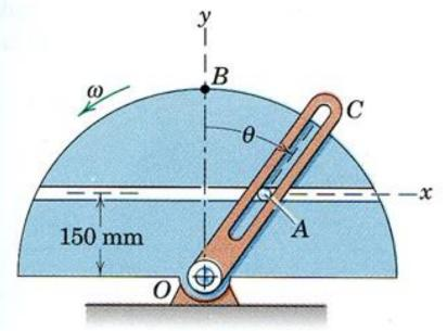
5/163 (4<sup>th</sup>), 5/168 (5<sup>th</sup>), 5/178 (6<sup>th</sup>), 5/176 (7<sup>th</sup>), 5/179 (8<sup>th</sup>) For the instant represented, link CB is rotating counterclockwise at a constant rate N = 4 rad/s, and its pin A causes a clockwise rotation of the slotted member ODE. Determine the angular velocity  $\omega$  and angular acceleration  $\alpha$  of ODE for this instant.
