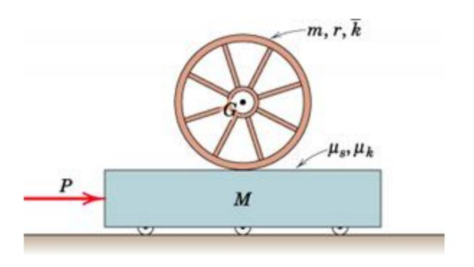
No-slip condition at the contact point P is:  $a_{P_t} = a_C$   $a_{P_t} = a_C = a_G + r\alpha$ ,  $\omega = 0$  Also for  $P_{max}$ ,  $F_f = \mu_s N$  For the disk:
