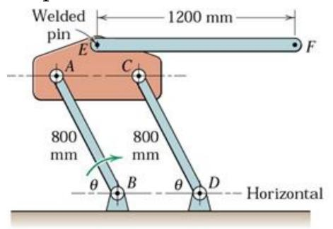
In a parallelogram linkage (which is a special type of a four-bar mechanism) the blue body that has no joint with the ground (coupler or floating link) is in translation.
