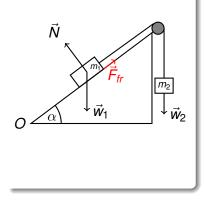
A mass  $m_1$  is on an inclined plane. A second mass  $m_2$  is attached to the first mass through a massless string and pulley system. The surface of the inclined plane has friction.
