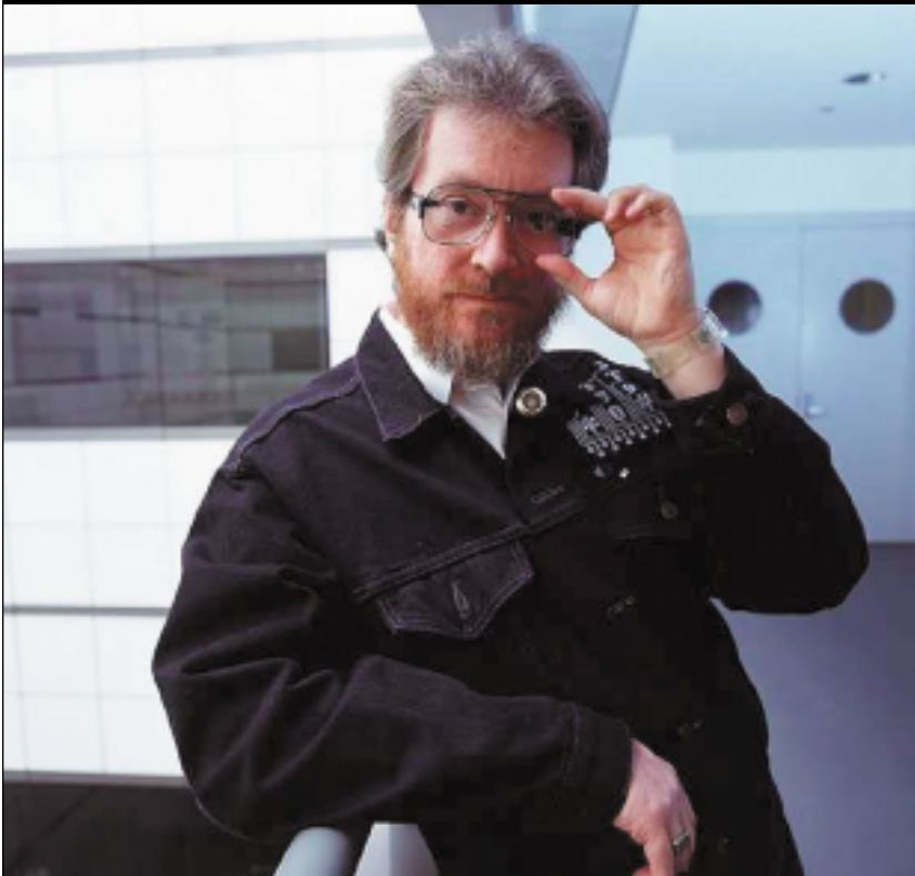
Figure 4. The author wearing a variety of new devices. The glasses (built by Microoptical, Boston) contain a computer display nearly invisible to others. The jacket has a keyboard literally embroidered into the cloth. The lapel has a context sensor that classifies the user's surroundings. And, of course, there's a computer (not visible in this photograph).
