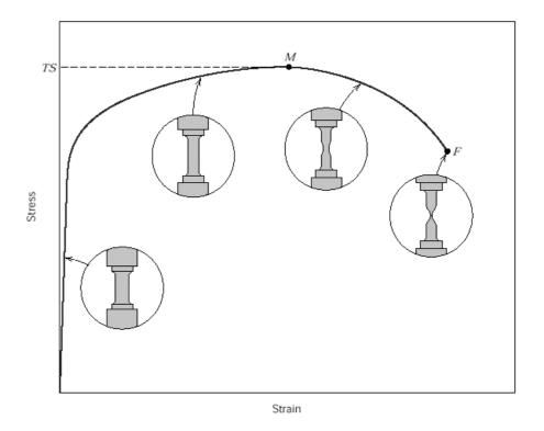
Typical engineering stress-strain behavior to fracture, point F. The tensile strength is indicated at point M. The circular insets represent the geometry of the deformed specimen at various points along the curve.
