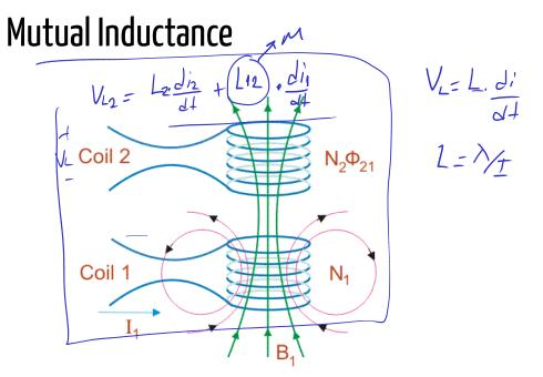
Write down the voltage equation of Inductor 2.
