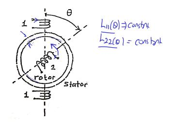
$$T=\underbrace{i_1i_2}_{\text{power}}\frac{\partial M}{\partial \theta}$$
