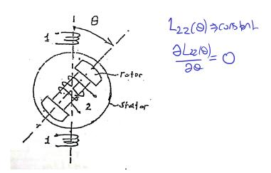
$$T = \frac{1}{2}i_1^2 \frac{\partial L_{11}}{\partial \theta} + \underbrace{i_1 i_2} \frac{\partial M}{\partial \theta} : (L_{22} \text{ constant})$$
