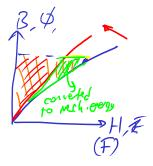
Electrical Energy = Magnetic Energy + Mechanical Energy
