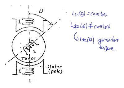
$$T = \frac{1}{2}i_2^2 \frac{\partial L_{22}}{\partial \theta} + i_1 i_2 \frac{\partial M}{\partial \theta} : (L_{11} \text{ constant})$$
