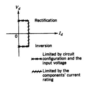
Capable of supplying negative Vd (Q4, Inversion)
