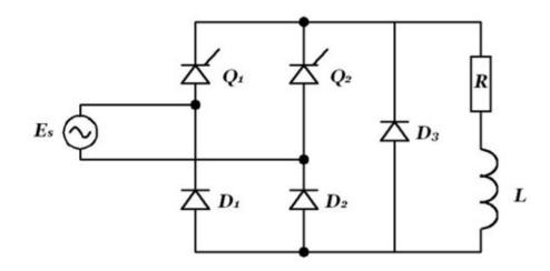
D3 can be removed (depending on load, and thyristor gate signals)
