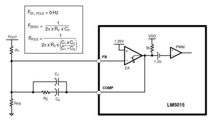
Figure 15. Type II Compensator
