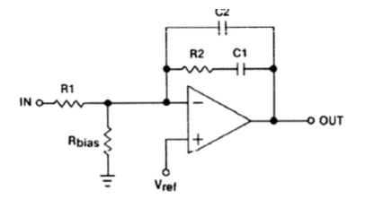
Figure 7. Schematic Diagram of a Type 2 Amplifier
