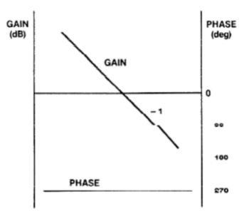
Figure 6. Transfer Function of a Type 1 Amplifier
