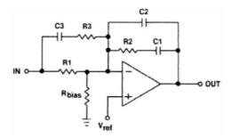
Figure 9. Schematic Diagram of a Type 3 Amplifier
