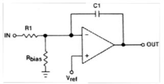
Figure 5. Schematic Diagram of a Type 1 Amplifier
