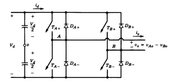
Voltage level is twice of the half bridge inverter
