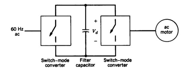
Back-to-Back Converter, Active Front-End Converter, Variable Frequency Drive (VFD)
