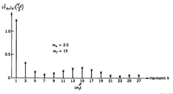
Figure 8-7 Harmonics due to overmodulation; drawn for  $m_a = 2.5$  and  $m_f = 215^{.50}$
