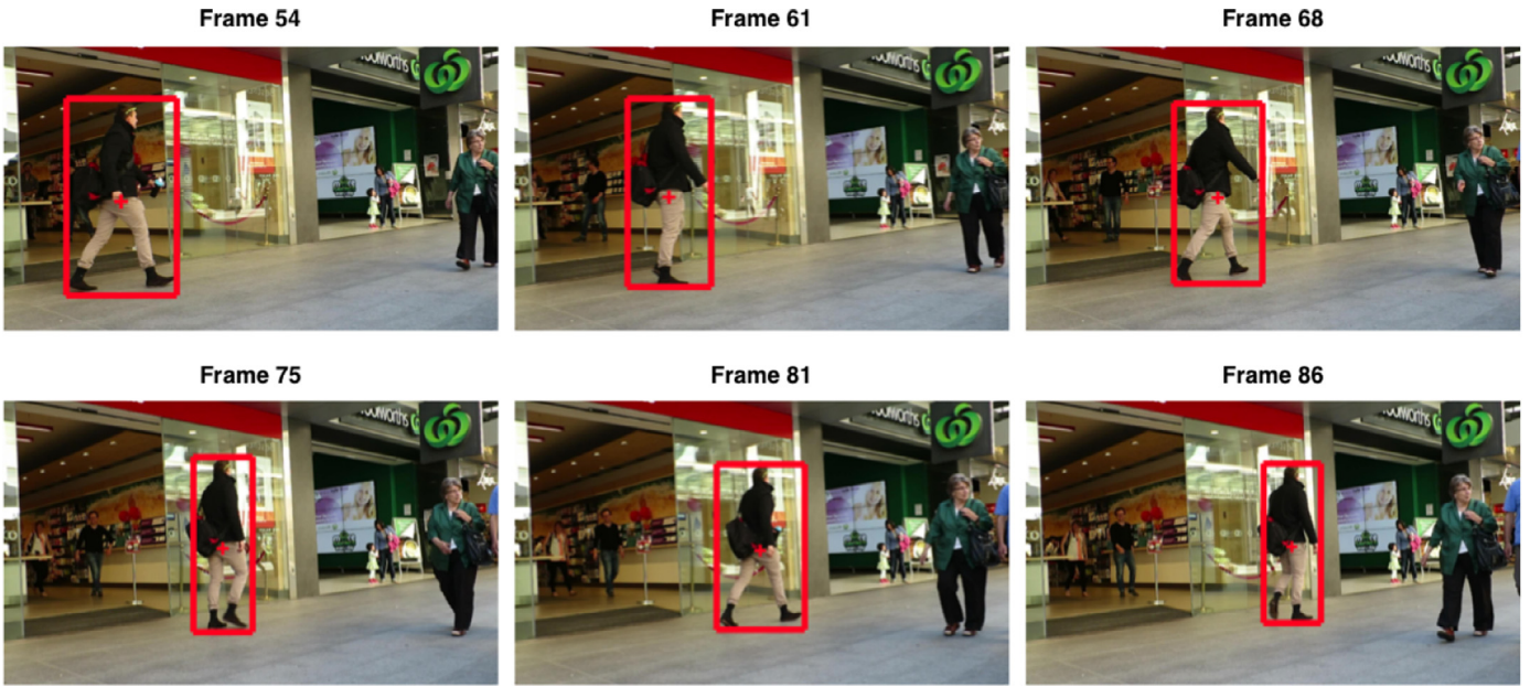
Fig. 7. The width of the detection bounding box changes periodically according to the changes of the walking pose (video sequence MOT16-10).
