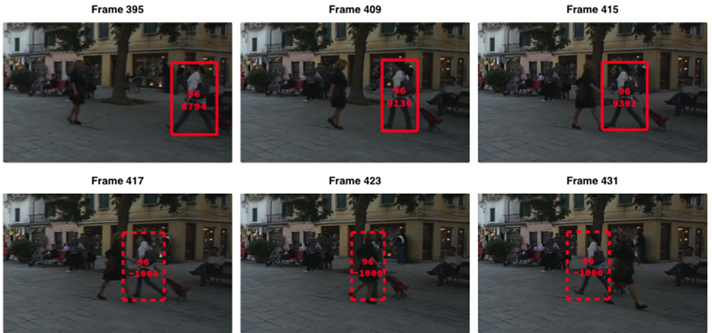
Fig. 10. Motion prediction using RNN in video sequence MOT16-01 from frame 395 to frame 431; (first row) actual track, (second row) bounding boxes with dashed line are the predicted detection bounding boxes by the RNN.
