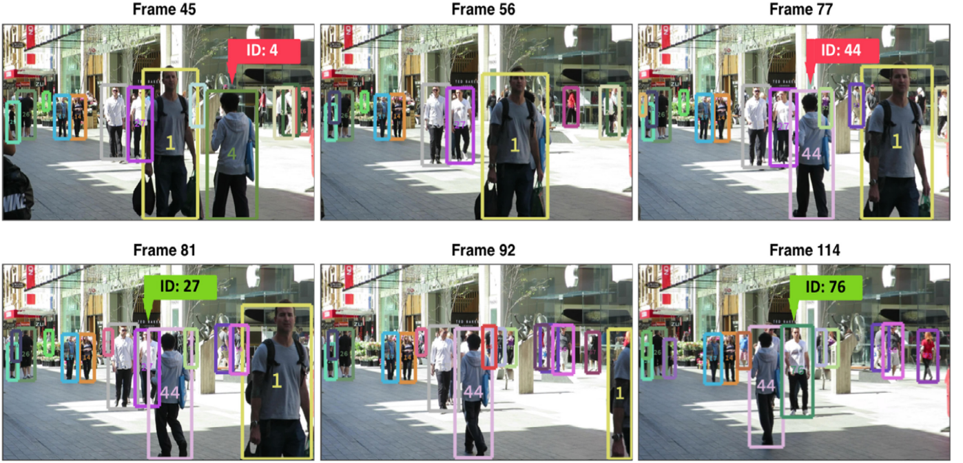
Fig. 4. Long-term occlusion. An example in video sequence MOT16-08 from frame 45 to frame 114, not handled by the lifted graph optimization. ID 4 and ID 44 belong to the same person but are occluded by ID 1. Similarly, ID 27 and ID 76 belong to the same person but are occluded by ID 44.
