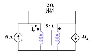
$\textbf{Question 3} \;\; \text{Find the input resistance} \;\; R_{\text{in}} \; \text{of the one-port circuit below}.$
