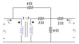
**b)** The secondary port is terminated with a 10  $\Omega$  resistor as shown below. Find the input resistance R by driving the port terminals with a test source.
