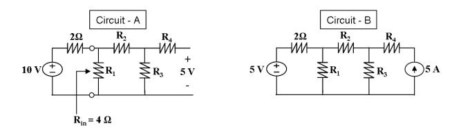
Find the power supplied/absorbed by the 5 V source in Circuit - B.
