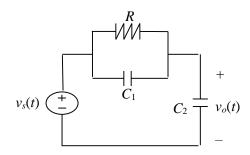
a) Find the zero-state response for  $v_0(t)$  for the input given below.
