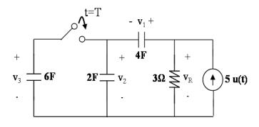
$v_1(0^-) = -6 V$ ,  $v_2(0^-) = 3 V$ ,  $v_3(0^-) = -1 V$ ;  $T = 4 \ln(3)$  sec.
