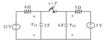
$v_{c1}(0) = -4 V$ ,  $v_{c2}(0) = -1 V$ ; T = 36ln(2) sec.
