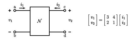
a) Is  $\mathcal{N}$  a passive or an active two-port? Why? <u>Hint:</u> Denote the resistance matrix by R. Write  $R = R_s + R_{ss}$  where  $R_s = (R + R^T)/2$  is a symmetric matrix and  $R_{ss} = (R - R^T)/2$  is a skew-symmetric matrix.
