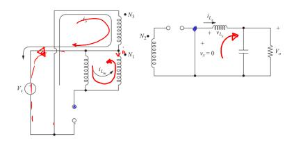
Lx feeds the load, Lm is discharged to the source:  $i_1 = -i_{Lm}$
