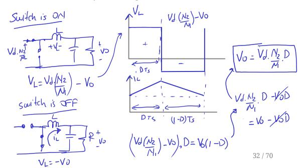
A buck converter with added turns ratio
