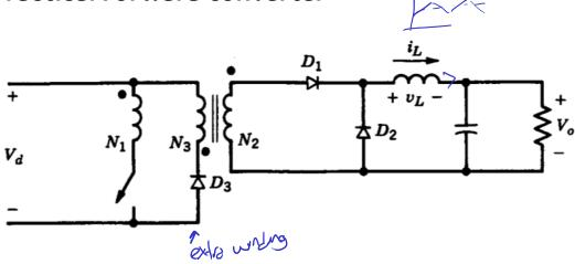
A transformer with two-primary windings
