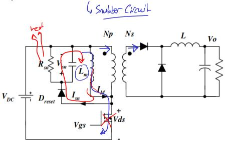
Magnetizing current dissipates through RCD circuit
