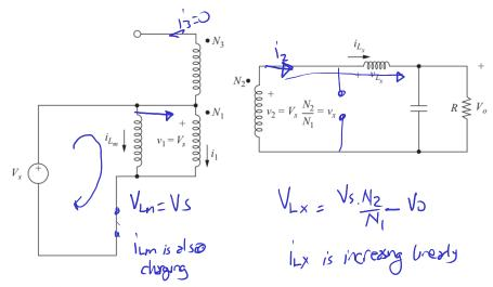
Lm is charged by input voltage, Lx is also charging
