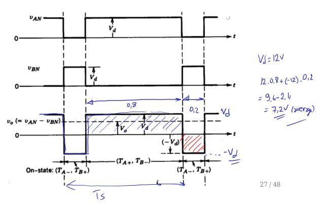
$$V_o = V_d \frac{v_{control}}{\hat{V}_{tri}}$$
