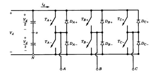
Three inverter legs are connected in parallel
