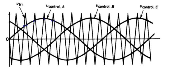
Vd or O voltage is generated at  $V_{AN}$  depending on the comparison.
