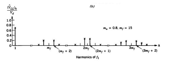
If mf is small, it is better to use synchronized PWM, and mf should be an odd interger, preferably multiple of 3 to reduce harmonics.
