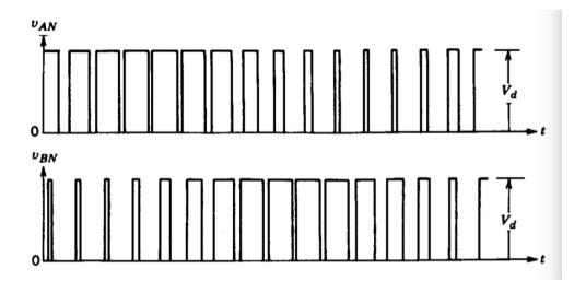
Line to line voltage ( $V_{AB} = V_{AN} - V_{BN}$ )
