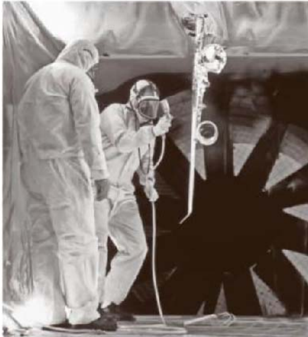
Fig. 4.12 PSP paint spraying in the covered test section itself
