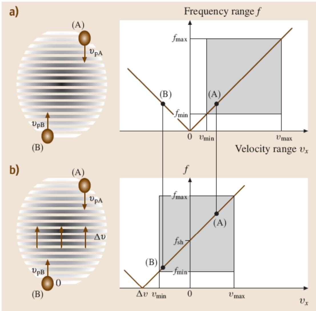
One further requirement is to distinguish the sign of the particle velocity, since the Doppler frequency alone does not contain this information as shown in **Figure (a)**. The same signal will be obtained for a particle crossing the fringes in either direction.
