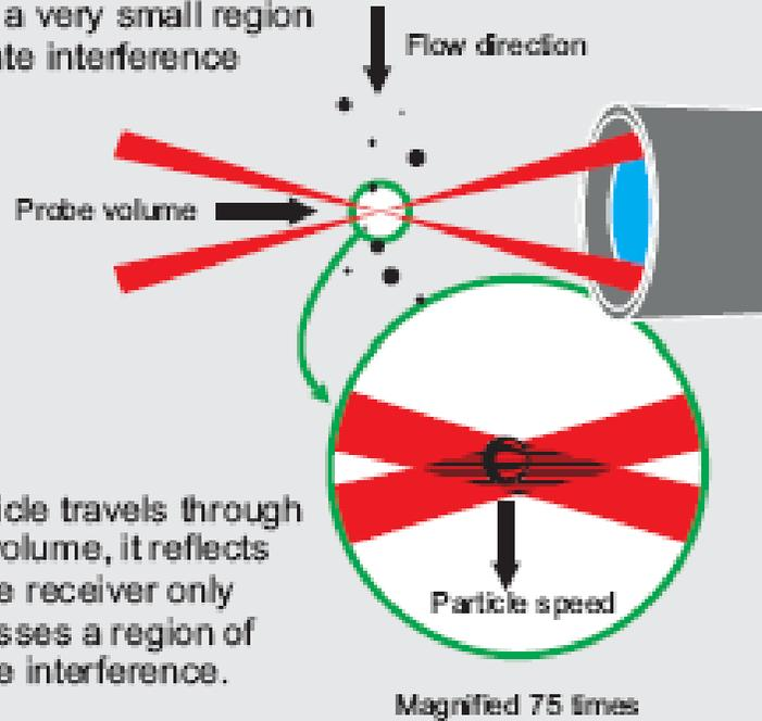
As the particle travels through the probe volume, it reflects light into the receiver only when it crosses a region of constructive interference.
