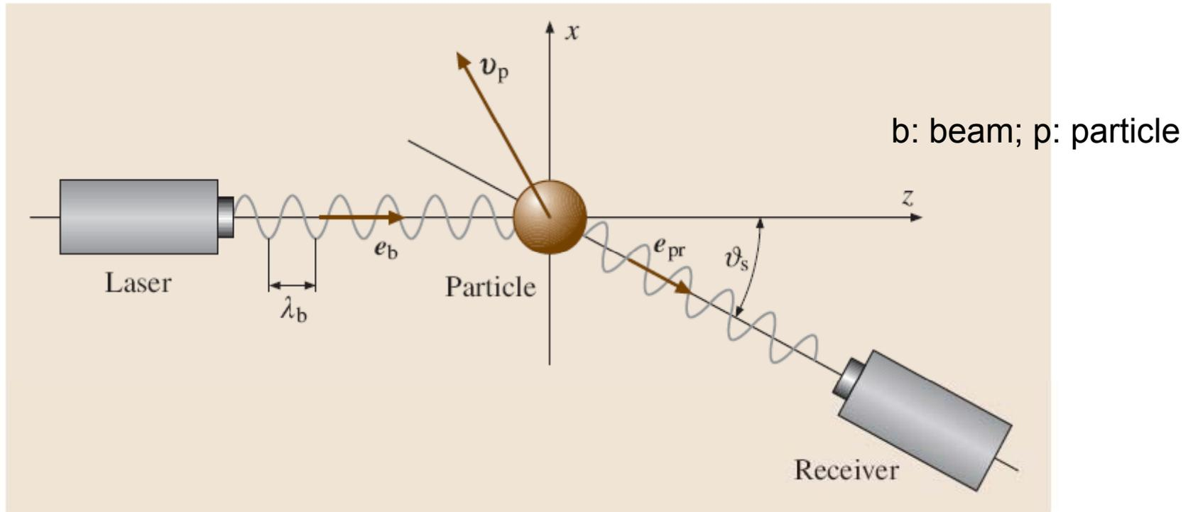
Defining geometry for applying the Doppler effect in the laser Doppler technique
