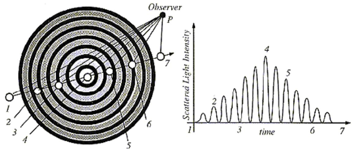
The interference pattern, known as a 'fringe' pattern is composed of planar layers of high and low intensity light. Velocity measurements are made when particles 'seeded' in the flow pass through the fringe pattern created by the intersection of a pair of laser beams.
