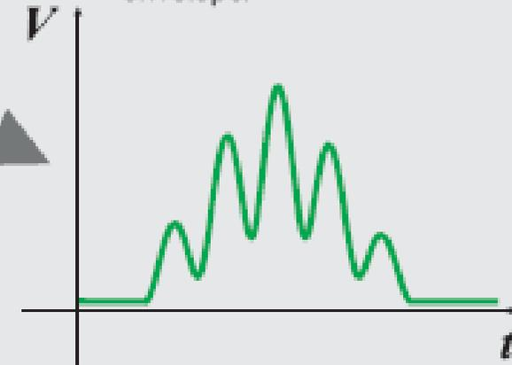
The sinusoid is isolated by a bandpass frequency filter.
