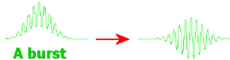
The **pedestal** is due to the intensity of the laser beam and usually has a Gaussian Distribution.
