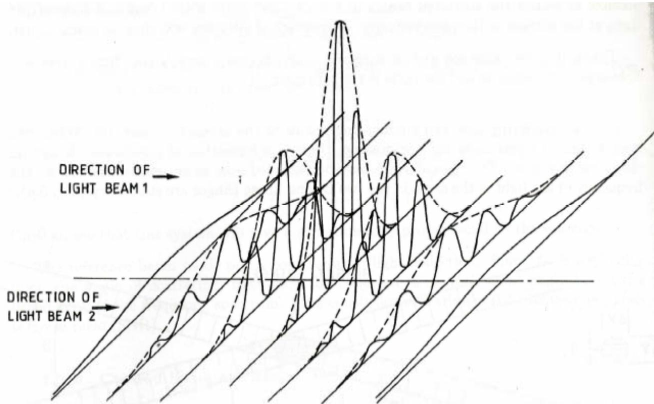
Figure 6.5: Sketch of light intensity distribution in the region of interference of two Gaussian light beams, assuming the angle between the two light beams is fairly small
