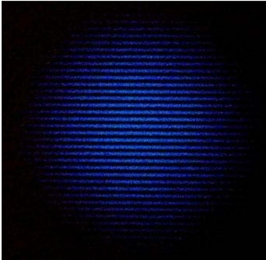
**This is an actual cross-sectional view of the beam crossing of two pairs of beams which illustrates a two component fringe pattern produced by an Argon-Ion Laser.**
