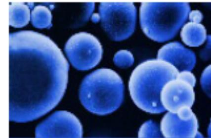
Hollow glass spheres and silver-coated hollow glass spheres (HGS & S-HGS)
