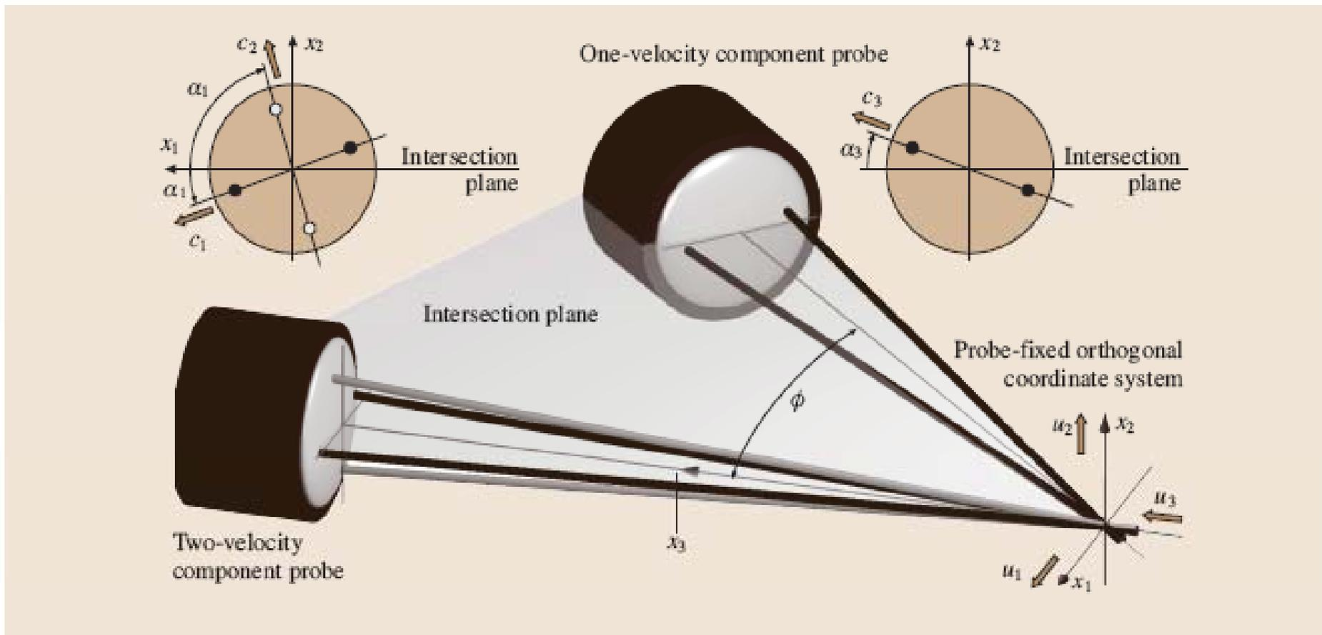
Three-velocity component laser Doppler system, showing measured velocity components and probe-fixed, orthogonal coordinate system
