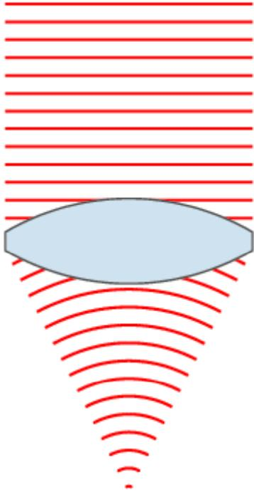
A lens can be used to change the shape of wavefronts. Here, plane wavefronts become spherical after going through the lens.
