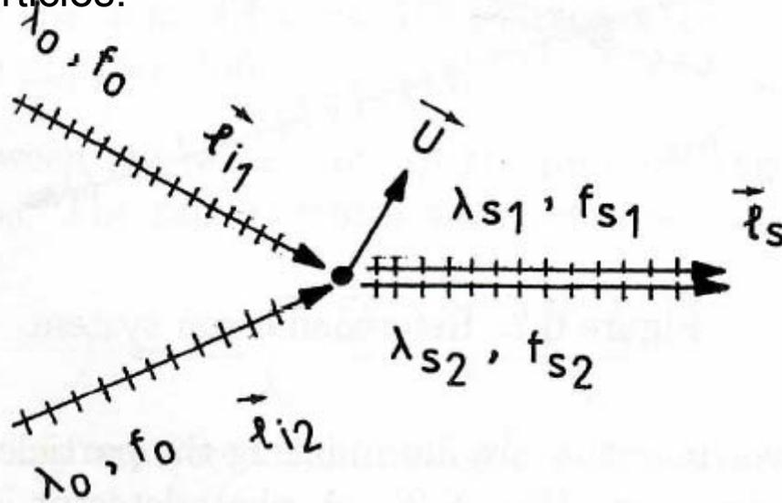
Each beam is scattered; this results into two beams  $(\lambda_{s1}, f_{s1})$  and  $(\lambda_{s2}, f_{s2})$  scattered in  $\vec{l}_s$  direction.
