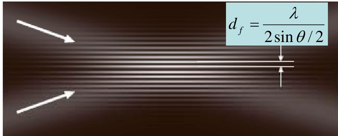
Interference pattern in the measurement volume
