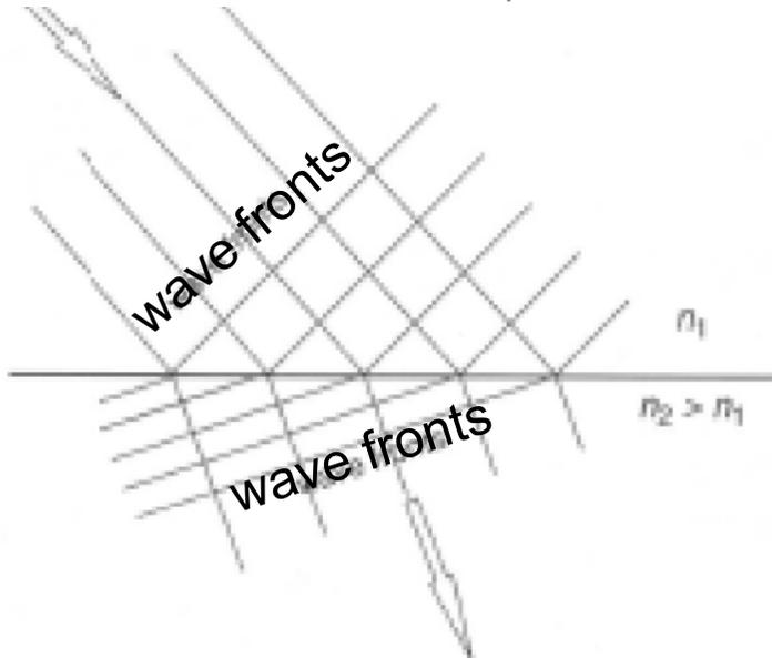
Interpretation of light refraction at the interface between two media as the rotation of wave fronts.
