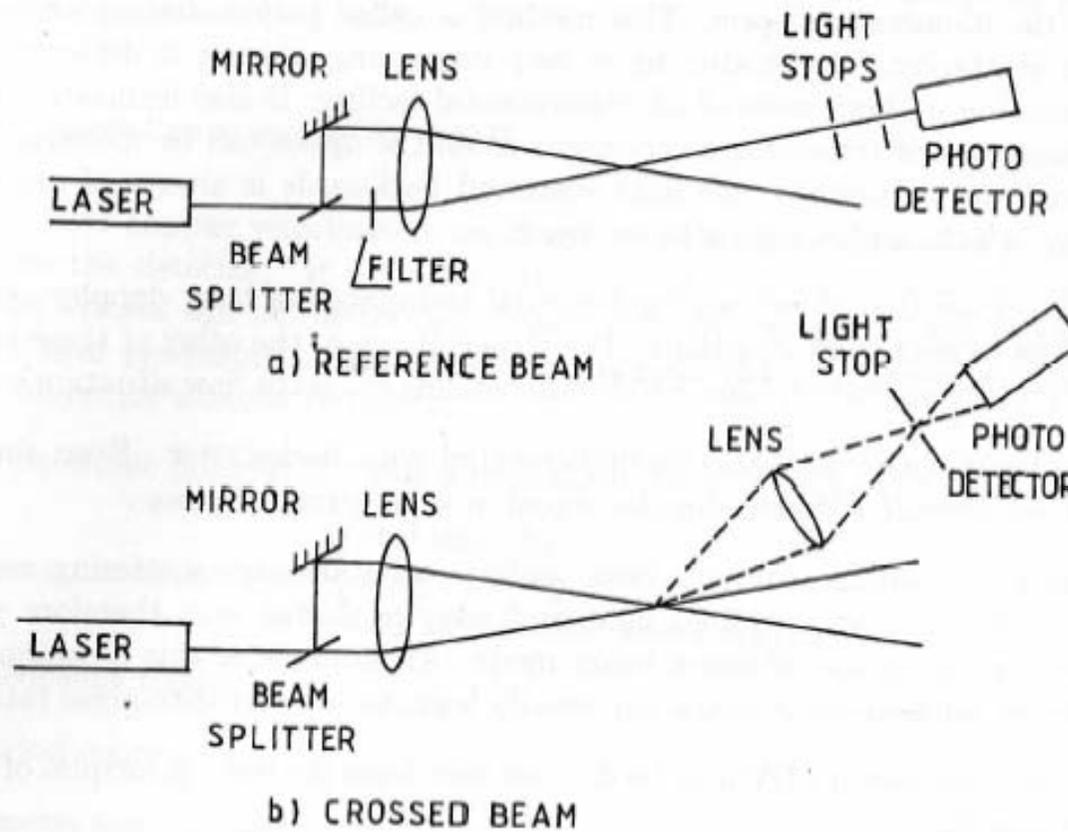
Figure 6.6: Different optical setup
