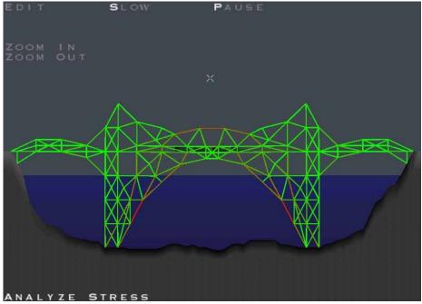
Bridge Builder also does a great job communicating the status of your structure during the simulation/test mode. Bridge segments are color-coded by the amount of stress they're under. It's an elegant way to show you which areas of your bridge are robust and which are likely to fail.
