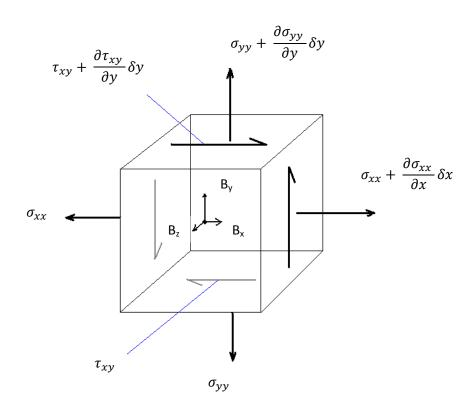
Normal and shear stresses on cubic infinitesimal element
