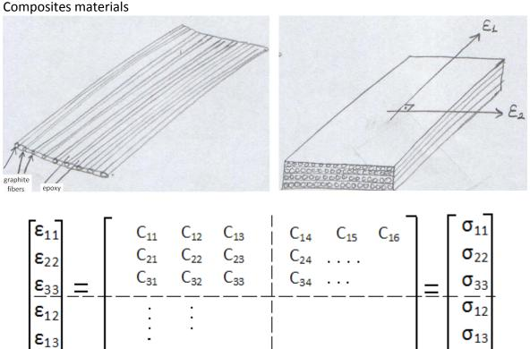
If there are axes of symmetry in 3 perpendicular directions, material is called **ORTHOTROPIC** materials.
