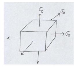
\* normal strains  $\begin{aligned} & \epsilon_x = 1/E ( \sigma_x - \nu(\sigma_y + \sigma_z) ) \\ & \epsilon_y = 1/E ( \sigma_y - \nu(\sigma_x + \sigma_z) ) \\ & \epsilon_z = 1/E ( \sigma_z - \nu(\sigma_x + \sigma_y) ) \end{aligned}$
