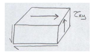
$\gamma_{xy} = \tau_{xy}/G$  (G: shear modulus)
