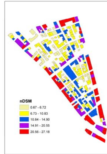
Figure 5. Average building heights calculated for each zone defined by building polygons in shape data retrieved from nDSM
