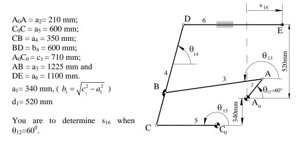
The loop equations, the equations that determine the relation between variable parameters due to the geometry of the mechanism, are given in terms of four nonlinear equations as:
